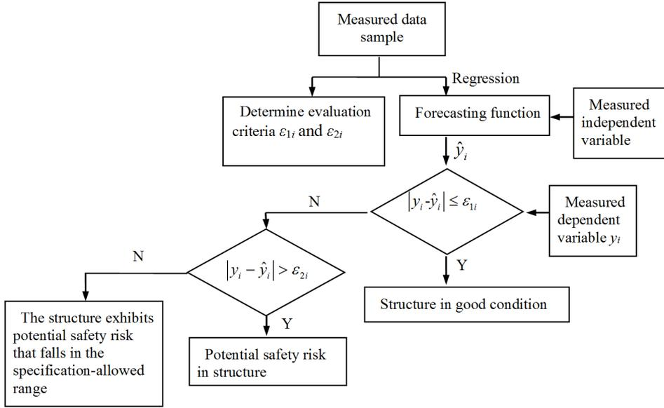
Fig. 1. Flow chart of forecasting function method
